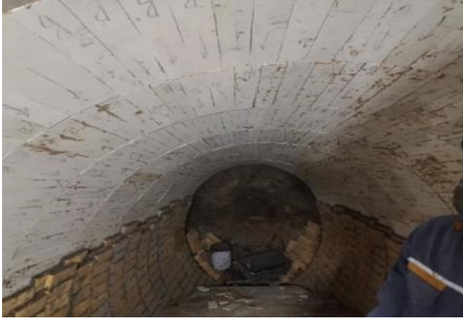
Figures 2 and 3 - Installed Superwool 1650SI Boards in torpedo ladle
