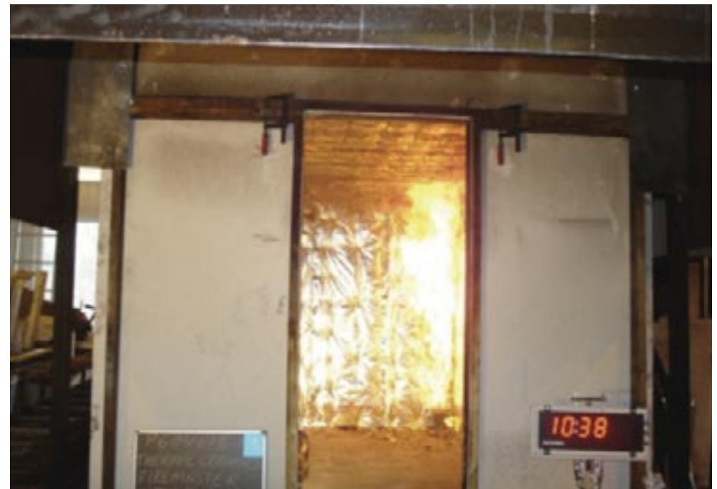
Room corner test in process showing the burner placed in the corner of the room
